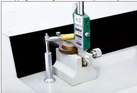
lapping measuring surfaces of caliper lower jaws
