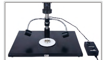
illumination direction and brightness are adjustable
